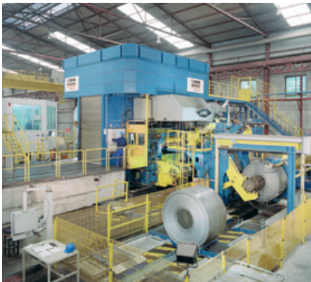
▲ Measuring the diameter of the coil enables the automatic change of the coil in automated production lines.
